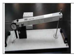
**Device Name**: Creep Measurement Apparatus.
